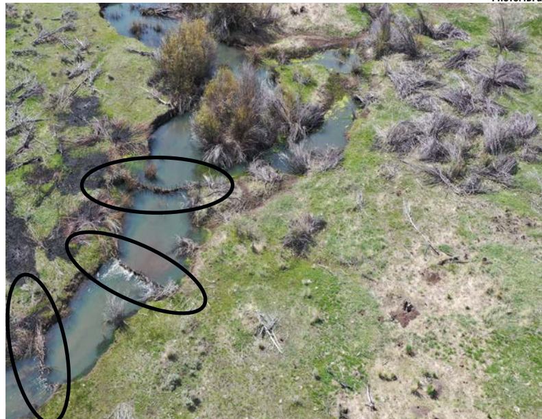
Below: The three BDAs in this complex are building up the streambed as well as forcing water into a neighboring side channel.
