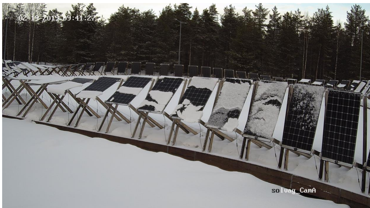
Figure 50: Snow wave, frameless bifacial modules, Piteå, N65, Sweden early spring 2019.
