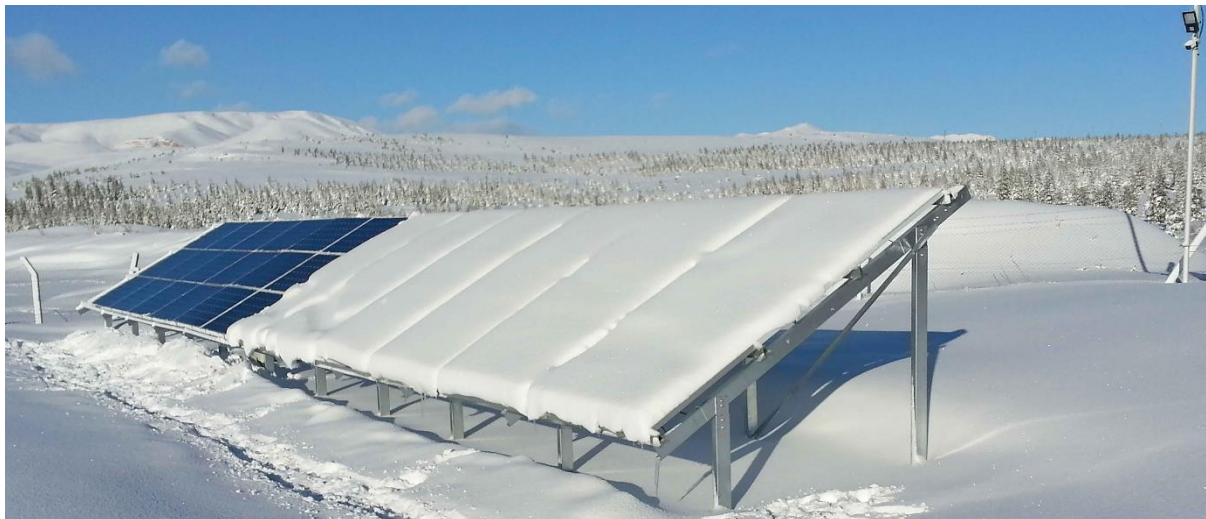
Figure 51: The system in Konya, Turkey, where one string was cleaned from snow every day at 09:00 AM [165].
