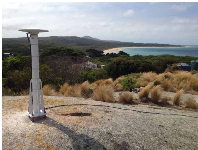
Land based global navigation satellite system (GNSS) reference station on Three Hummocks Island that forms part of IMOS' satellite calibration and validation infrastructure.
