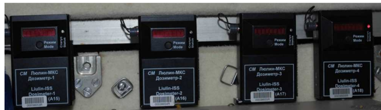
Fig. 2. The 4 active Liulin-MKS dosimeters at Russian Segment of ISS. Picture was taken on 3 rd of March 2011 by Russian Astronaut Kondratiev.
