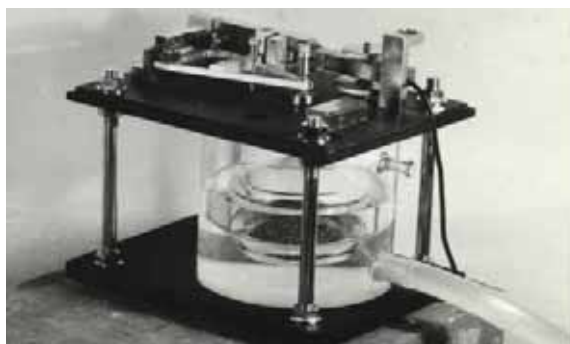
Figure 2. Water-tube tiltmeter (single terminal)
