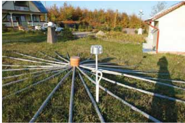
Figure 3. The Chaparal infrasound sensor located at Plostina main building (PLO4)
