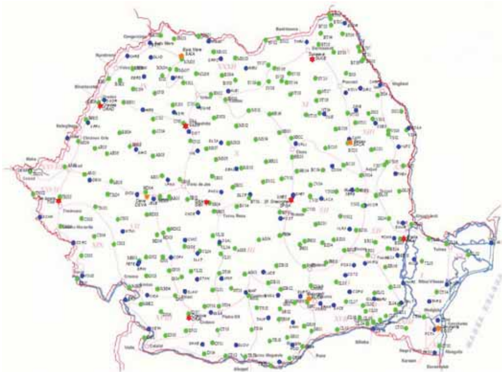
Figure 3. Class B - National Spatial Geodetic Network (NSGN) (green – new monuments; blue – old monuments from triangulation network)
