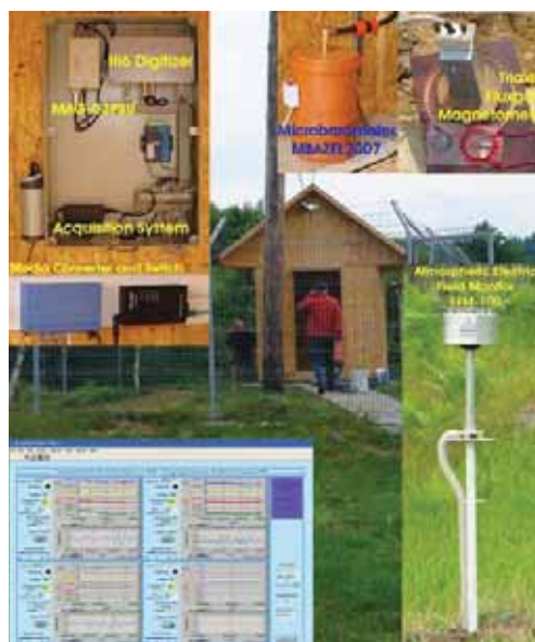
Figure 2. An outer image of PLO3 site and some of the equipments that are involved in the monitoring process: Data Acquisition System, Microbarometer MBAZEL2007, Triaxial Fluxgate Magnetometer MAG-03MS. However, the Electric Field Monitor EFM-100 is installed at PLO4, in the vicinity of the Weather Station WS-3600.
