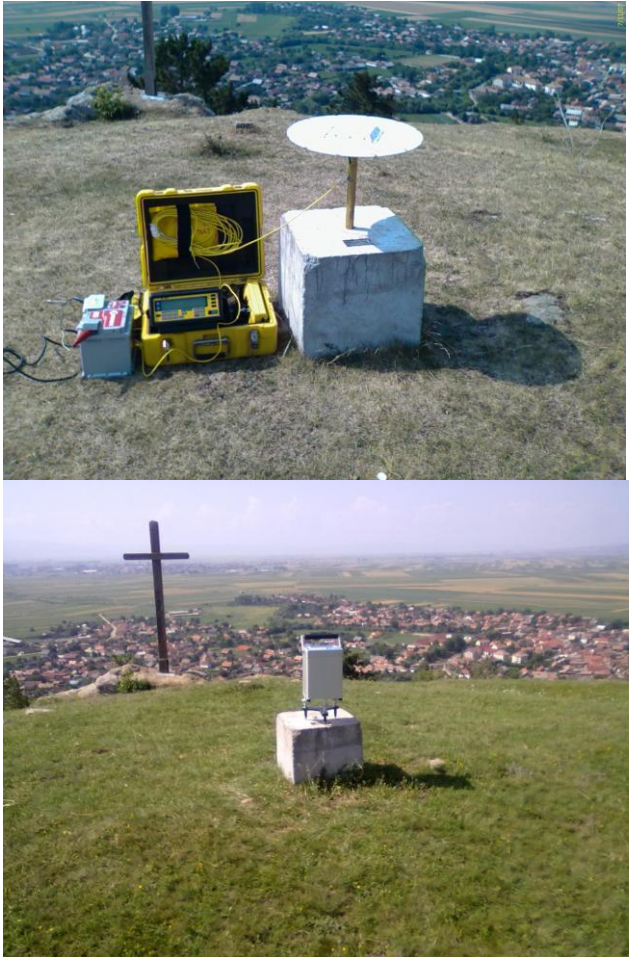
Figure 21. High accuracy GPS (left) and gravity observations (right) run on the P115 (Sanzieni) pillar of NGDN
