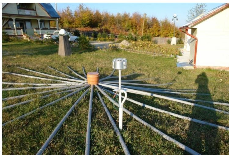
Fig. 3. The Chaparal infrasound sensor located at Plostina main building (PLO4)
