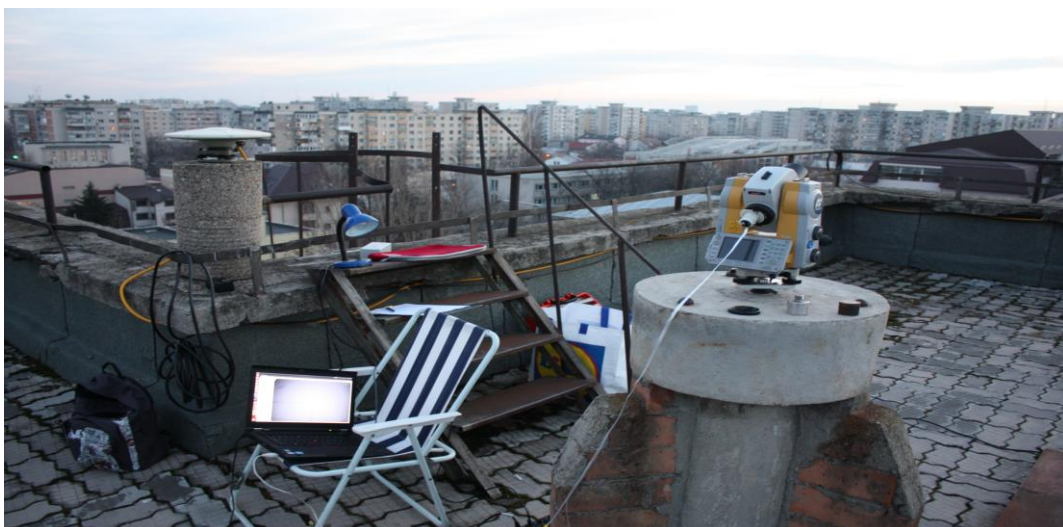
Figure 17. Astro-geodetic observations for vertical deviation determination
