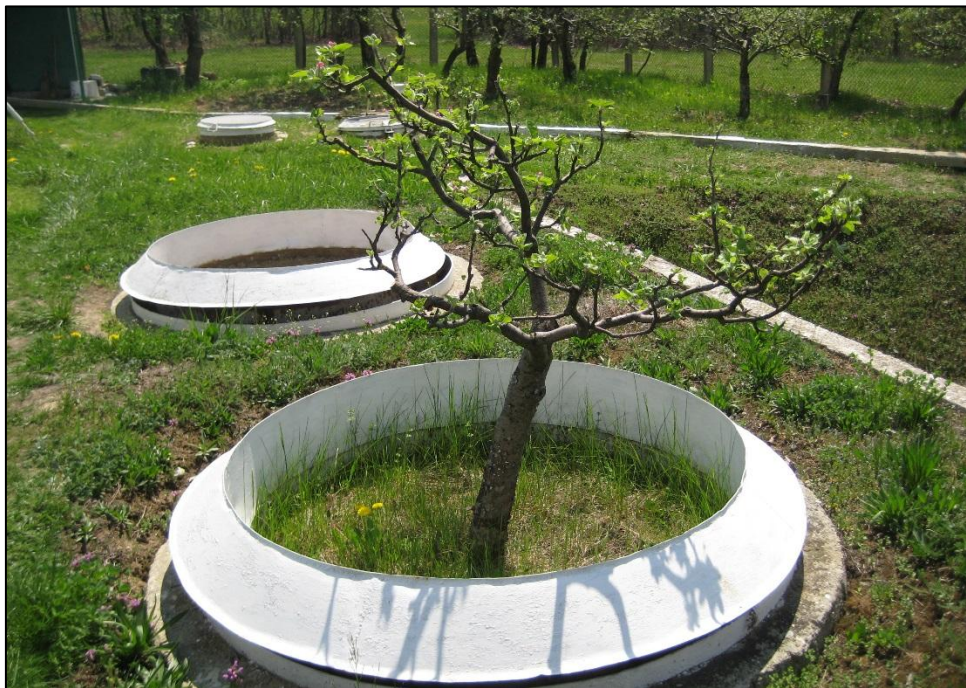
Figure 29. Lysimeter network at Voinești station
