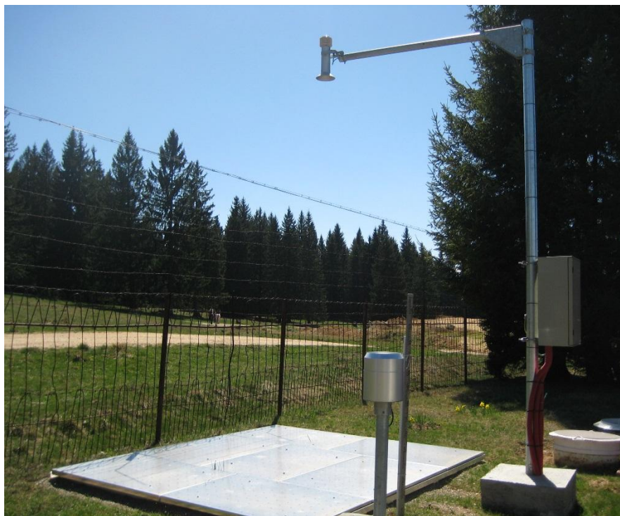
Figure 47. Automatic snow station at Poiana Brasov
