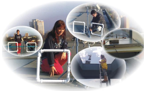
Fig. 5. Magnetic VLF and LF antennas installed on the roof of the Dobrudja Observatory
