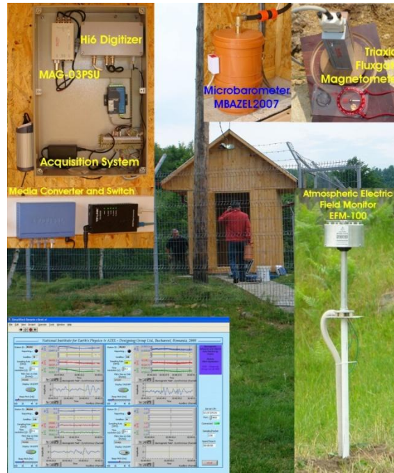
Fig . 2. An outer image of PLO3 site and some of the equipments that are involved.in the monitoring process: Data Acquisition System, Microbarometer MBAZEL2007, Triaxial Fluxgate Magnetometer MAG-03MS. The Electric Field Monitor EFM-100 is installed at PLO4, in the vicinity of the Weather Station WS-3600.
