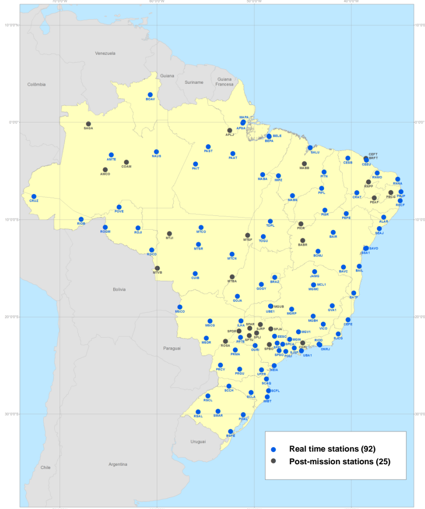
Fig. 2.2 The Brazilian Network for Continuous Monitoring of GNSS (RBMC)
