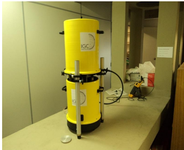
Fig. 2.5 Absolute gravity meter A10-32
