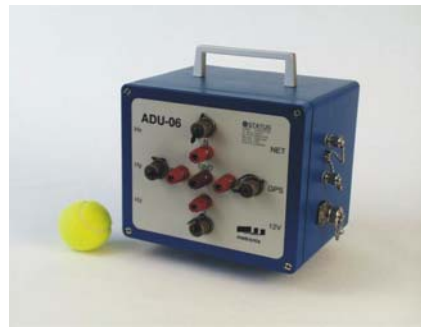
Fig. 7. ADU 06 with 5 channel (2 electric and 3 magnetic), GPS, flash memory, 24 bits resolution
