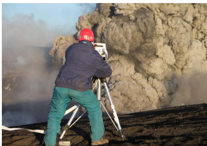
FTIR remote sensing of magma degassing from Eyjafjallajökull crater rim in May 2010, Iceland
