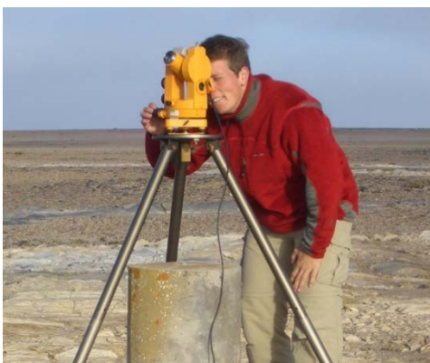
Measuring the geomagnetic field at a so-called repeat station in Namibia
