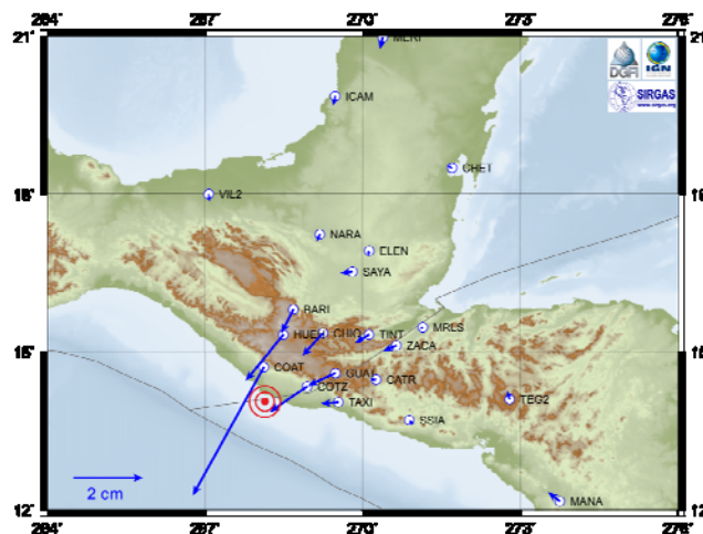
Horizontal displacements of the SIRGAS Reference Frame estimated after the 2012-11-07 Guatemala M7.4 earthquake
