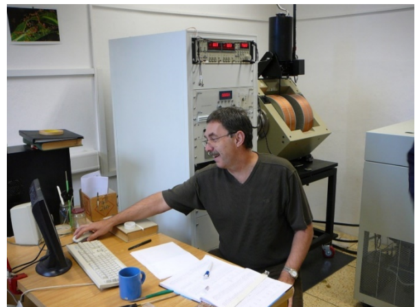
Measuring magnetic properties of rocks
