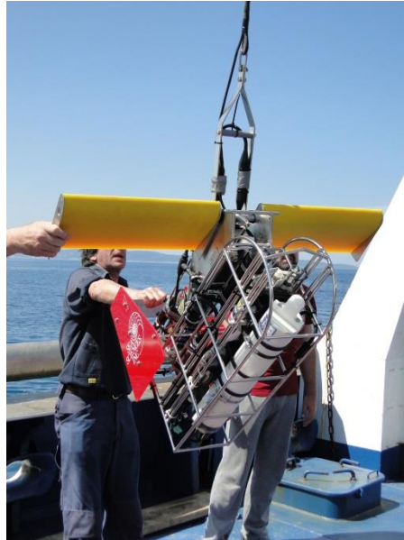
Figure 2. Deployment of towed undulating vehicle for high-resolution CTD profiling along a transect between Jabuka and Blitvenica (eastern middle Adriatic), in June 2019 (photo by Hrvoje Mihanović).
