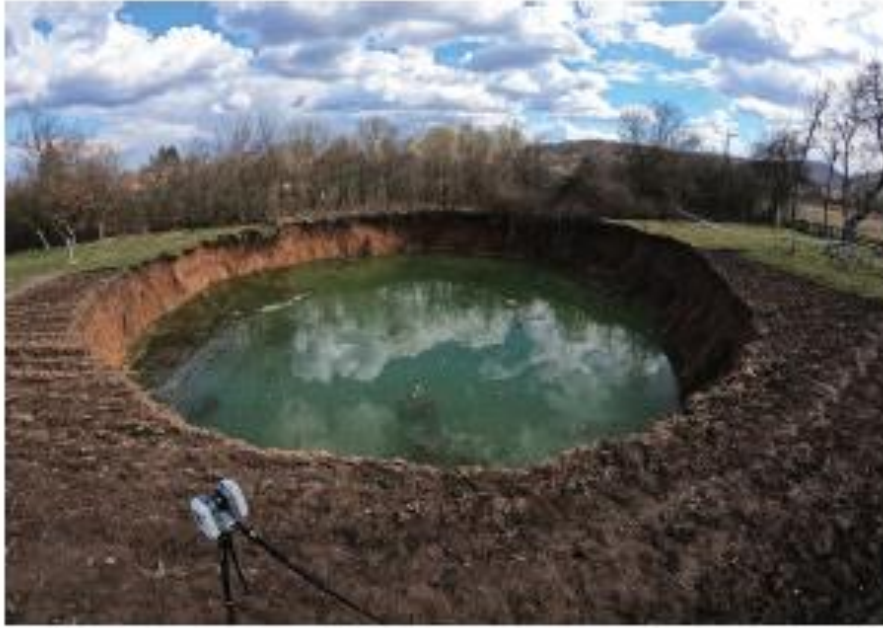
Figure 18. The largest sinkhole in Mečenčani village (diameter is 24.55 m) (from Tomac et al., 2022).
