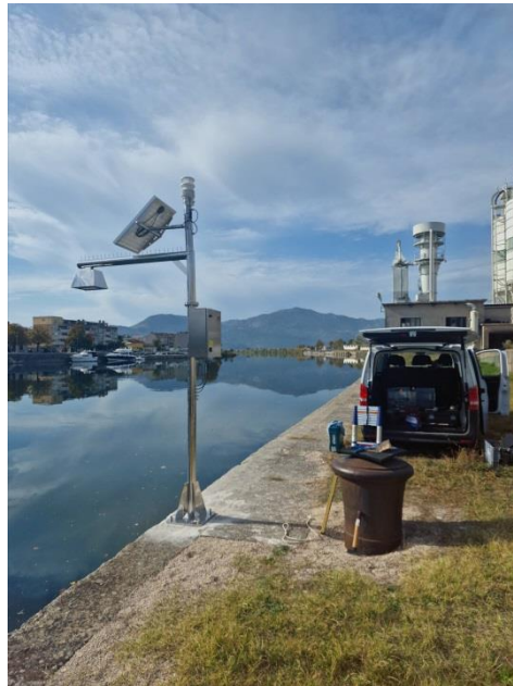
Figure 1. Meteo-oceanographic station being installed at Metković in the Neretva River estuary, in November 2022 (photo by Stipe Muslim).
