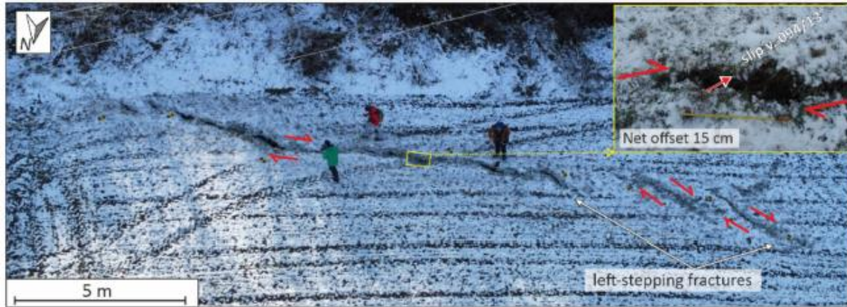
Figure 17. Aerial view (drone survey) of a \sim 20 -m-long surface rupture on alluvial fan gravels mapped southwest of Križ Hrastovački (from Baize et al., 2022). Surface faulting occurred as a continuous rupture, striking 120^\circ , or as a set of left-stepping en échelon ruptures. The maximum coseismic offset, measured between well-preserved piercing points, is \sim 15 cm.
