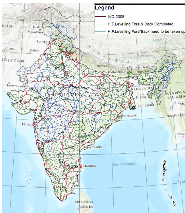
Figure 2: Levelling Network for Redefinition of Indian Vertical Datum
