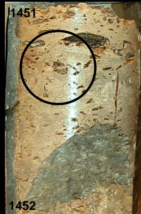
Vuggy porosity in the LG&E Wainscott #1 Oldham County, KY 1452-1453 ft
