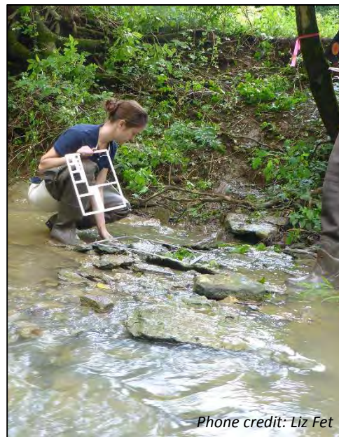
Figure 6-3: Conducting a pebble count as part of a hydromodification survey
