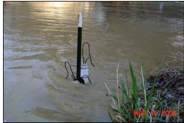
Passive High-Flow Stage Sampling Device
