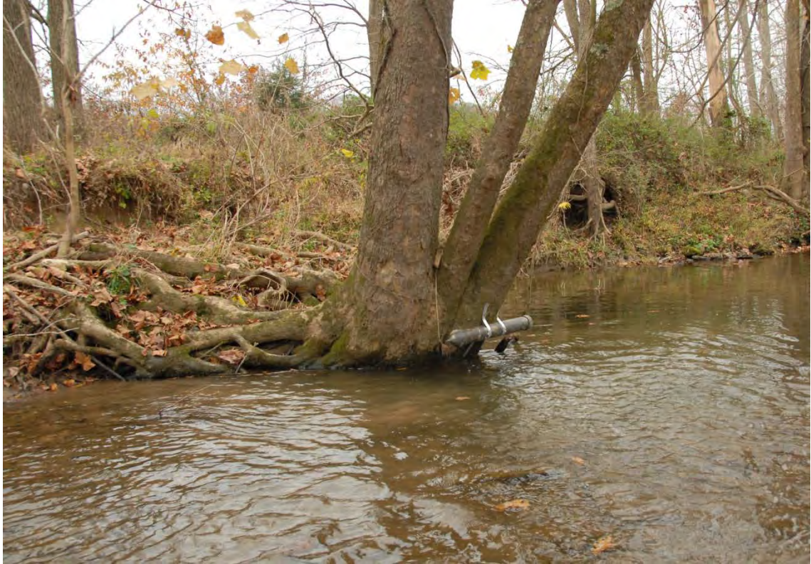
Figure 3.2 Passive sediment samplers were used to collect suspended sediment during flood events.
