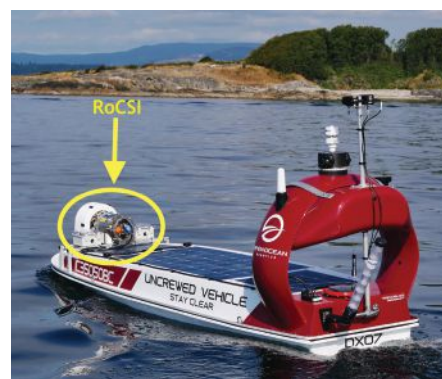
➤ McLane RoCSI eDNA sampler with 24 sample cartridge filter holders integrated with DataXplorer USV. (Credit: Open Ocean Robotics)
