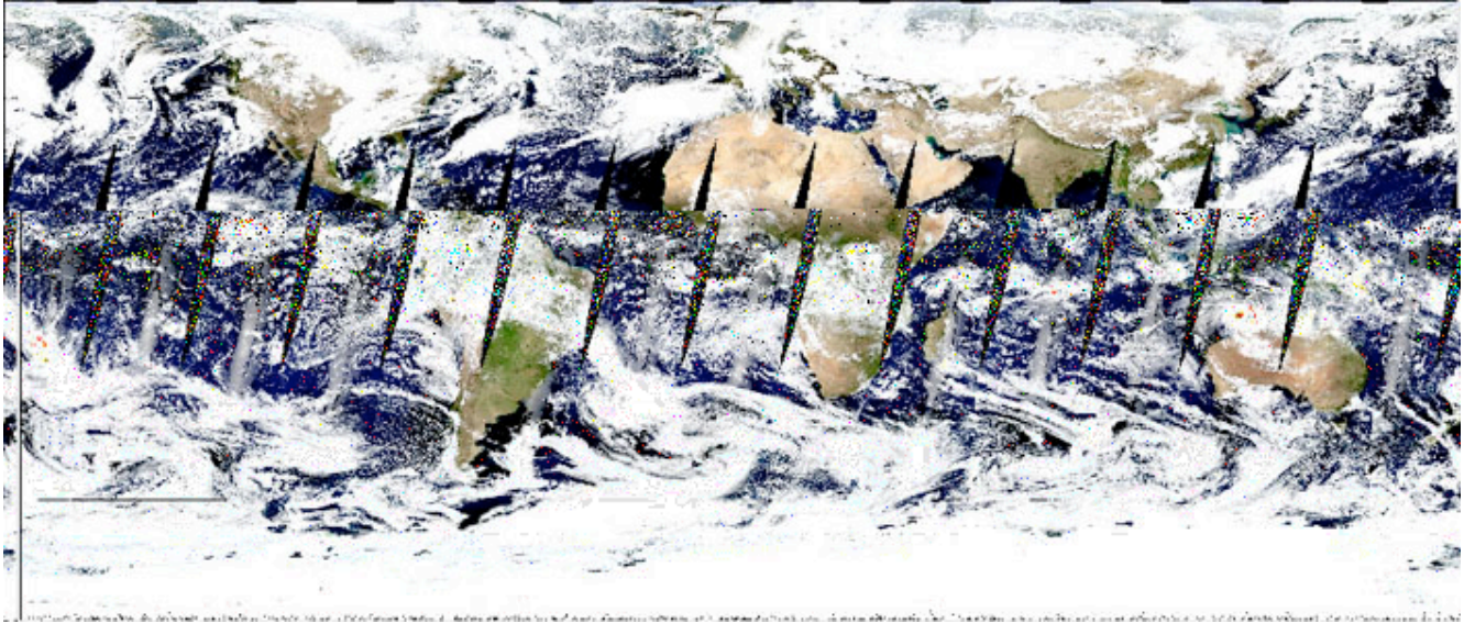
Figure 8. A MOD09CMG RGB-image composed of surface reflectance data measured by bands 1 (red), 4 (green) and 3 (blue) on December 7, 2000. The MODIS product granule ID is MOD09CMG.A2000341.005.2006347161131.hdf.
