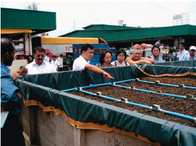
Figure 2 The public market was also the demonstration site of the use of "coco-peat" for wastewater filtration
