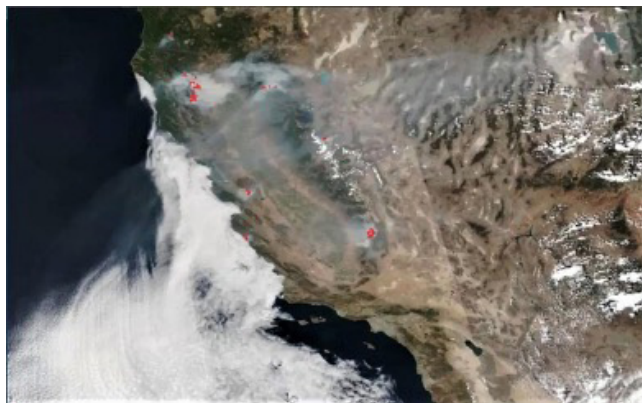
The VIIRS instrument captured the image above on August 30, 2020. It shows heat signatures (red dots) from several fires as well as clouds associated with a cooler marine layer just offshore the central and southern California coastlines.
