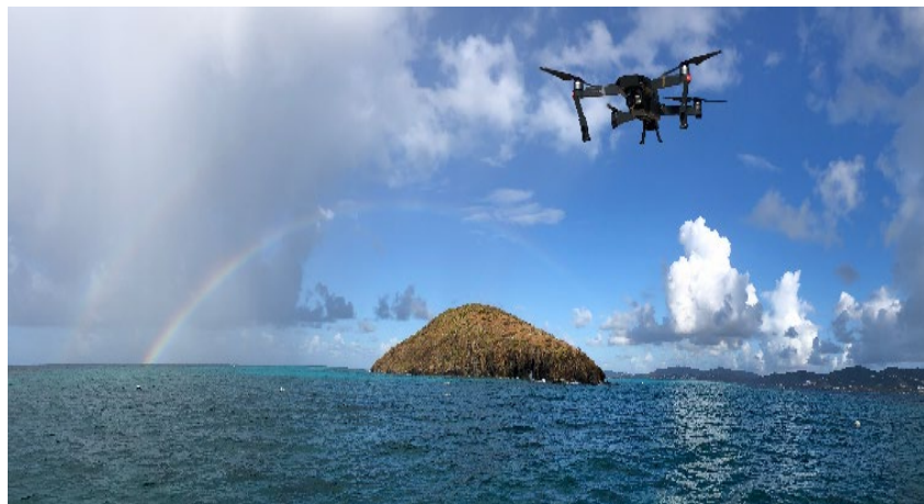
A small Unmanned Aircraft System (DJI Mavic Pro) flying east of Buck Island, St. Croix, USVI provides coastal mapping and elevation data for improved marine ecological and modeling. (Photo Credit: Oregon State University.)
