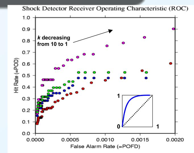
A more complicated shock monitor tests for changes in ACE solar wind velocity (V), density (D), total field (B) and component of velocity normal to the shock front (V.n). For dV/Vsigma=4; d(V.n)/(V.n sigma)=2; For dD/Dsigma=1.5; dB/Bsigma=2.5 we obtain POD=0.3 and POFD=0.00002. This POFD is equivalent to one false shock report per month on average.
