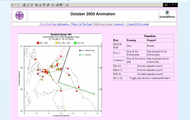
Upper Left: Grid GIC from network model, shown as geographic plot (also available as grid schematic map). Move cursor over plot to view individual station GIC (on right), with 95% confidence limits and with data estimated by accurate transfer function technique (see box below). October 2003 storm is shown. Upper Right: Animation of network GIC output for last hour. Snapshot from October 2003 storm shown.
