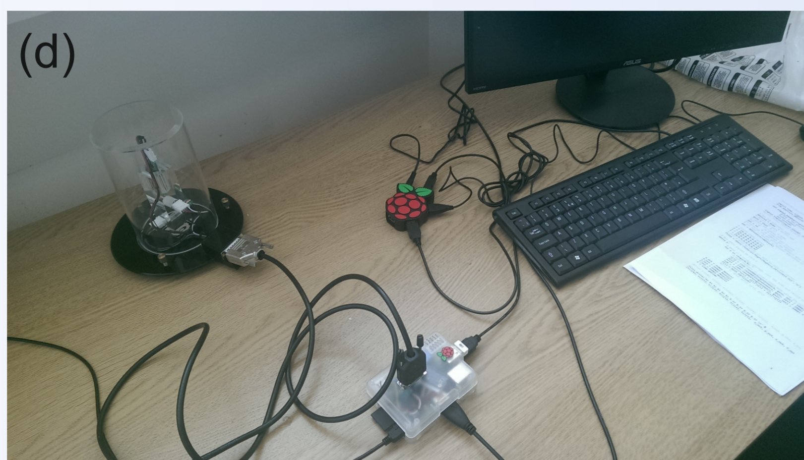
Figure 2: (a) Three FLC100 magnetometers from Stefan Mayer Instruments are mounted (b) orthogonally (North, East and Down) into a perspex block and wired together to common power and ground. The FLC100 magnetometers output a voltage proportional to the strength of the magnetic field. The output voltage is digitised by (c) an AB Electronics 17-bit digitiser connected to a Raspberry Pi computer. Software written in Python is used to read and record the values of the magnetic field from each component.
