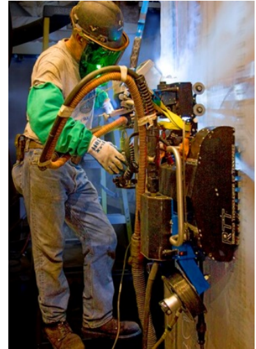
A worker uses the robotic welder. Credit: Jack Leustig, Steve Glovksy, and Mike Nutter, Bath Iron Works Photographer
