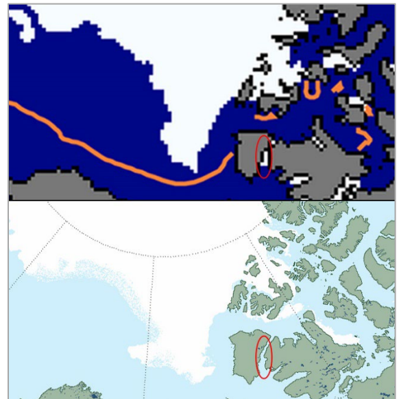
Figure 22. Screenshots of the Sea Ice Index daily extent (top) and MASIE daily extent (bottom) from 08 September 2011. The red ellipses show one area, between Banks Island and Victoria Island, where SII and MASIE differ significantly. MASIE is the more accurate product because of the visible band data used as input.
