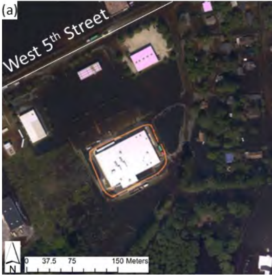
Figure 2-10. Examples of visible individual-level mitigation efforts in Lumberton implemented before the 2018 Flood; (a) Temporary perimeter flood protection around international retailer building (NOAA 2018); (b) Elevated air conditioning condensers in a public housing complex.
