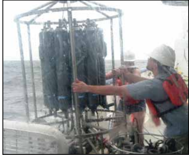
Researchers retrieve the CTD rosette, used for collecting water and measuring dissolved oxygen and other oceanographic parameters, after a sampling profile is completed during rough seas. Photo: L. Jewett, NOAA
