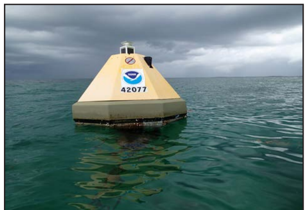
An ocean acidification buoy at Cheeca Rocks, an inshore patch reef within the Florida Keys National Marine Sanctuary. Credit: NOAA
