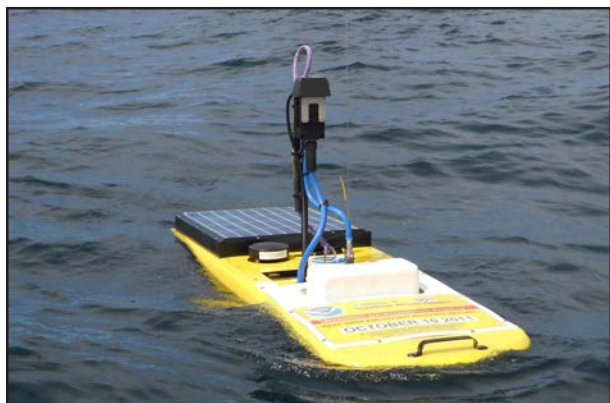
A wave glider makes ocean carbon dioxide ( p\text{CO}_2 ) measurements in Washington coastal waters while deployed by researchers aboard the R/V Wecoma . Credit: Richard Feely/NOAA
