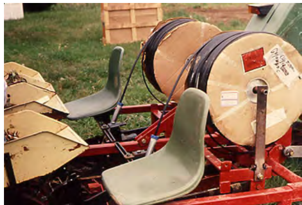
Figure 3-7. A two-chambered trickle irrigation tube can be automatically placed underground at the root zone in transplanting.
