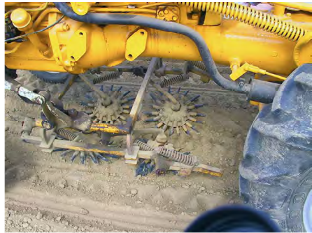
Figure 3-4-B. Close up of the Buddingham weeding machine showing plastic “fingers” on the rotating wheel.
