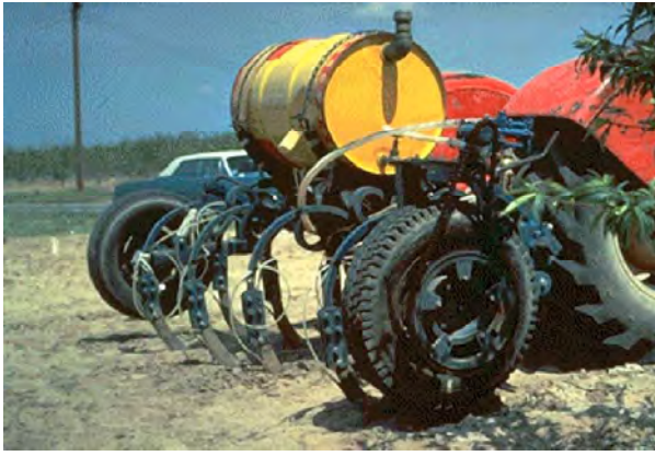
Figure 4-1-A. A gravity flow rig on a tractor for injecting liquid fumigants into the soil.
