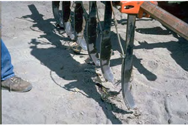
Figure 4-1-B. Shanks for injecting fumigants into the soil.
