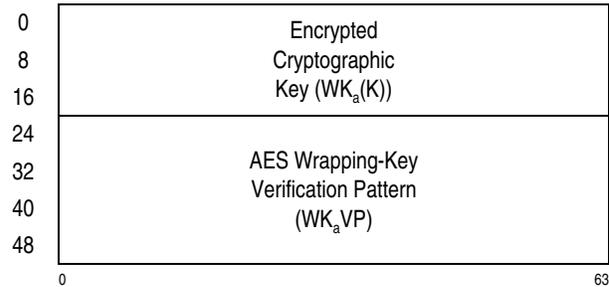
Figure 7-32. Parameter Block for KM-Encrypted-AES-192
