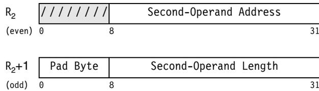
In the 31-bit addressing mode, the operand addresses would be in bit positions 1-31 of the even registers shown above.
