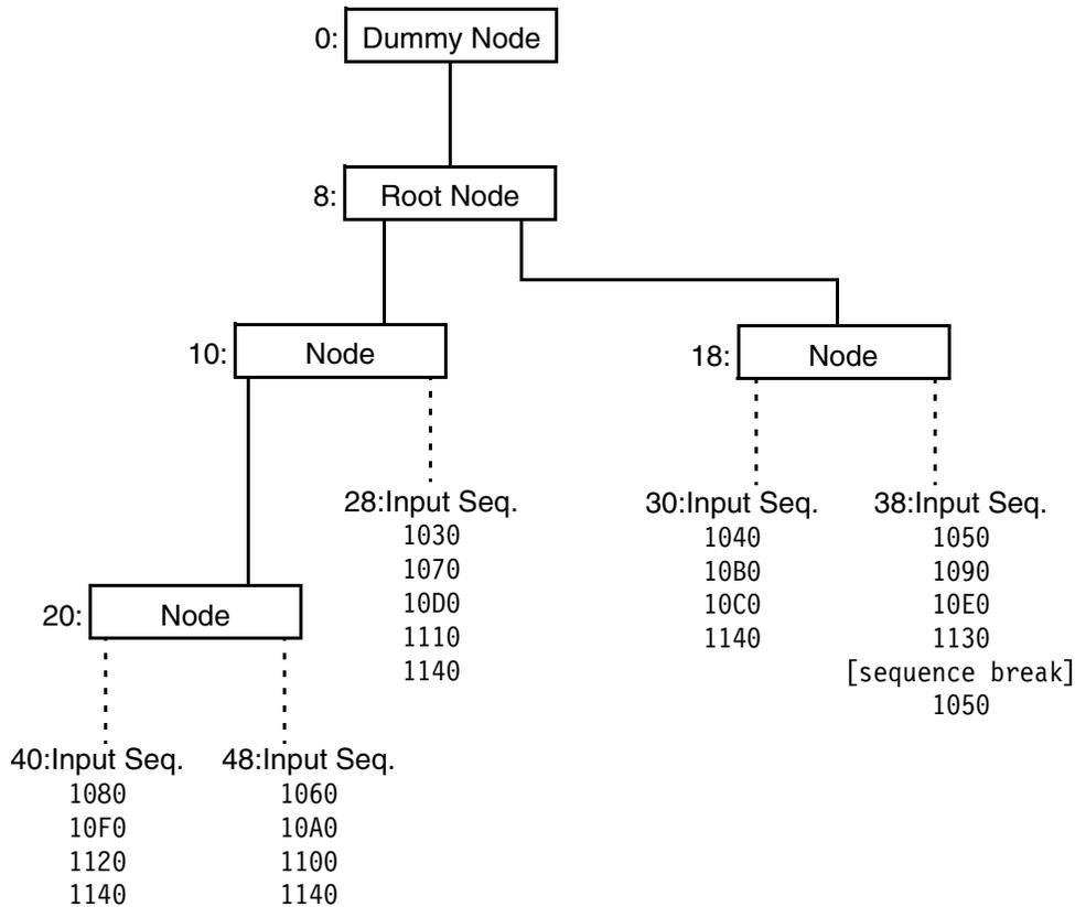
**Note:** Each node and input sequence is identified by a number which is the hexadecimal node index. Each input sequence is given as a list of record addresses (also in hexadecimal).
