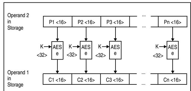
Figure 7-37. KM AES Encipher Operation Using 256-Bit Key
