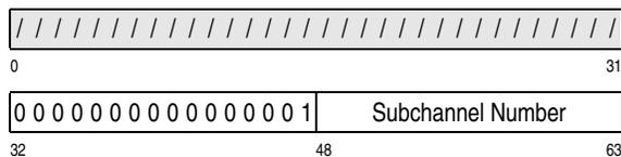
Bit positions 48-63 of general register 1 contain the binary number of the subchannel to be used for the function specified by the instruction. Bit positions 0-31 of general register 1 are ignored and bits 32-47 specify the binary number one.
