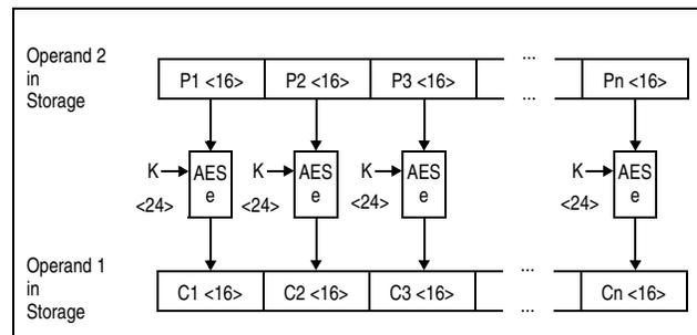
Figure 7-33. KM AES Encipher Operation Using 192-Bit Key
