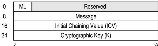
Figure 7-314. Parameter Block for PCC-Compute-Last-Block-CMAC-Using-DEA
