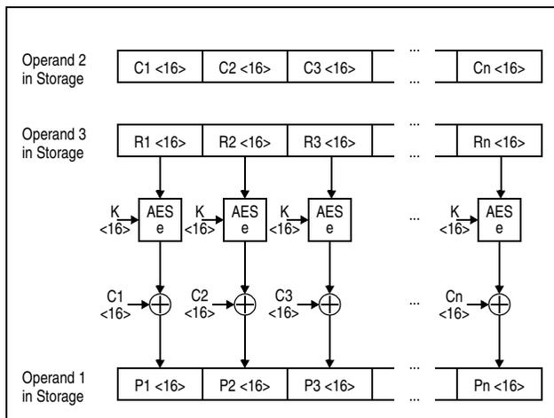
Figure 7-148. KMCTR AES Decipher Operation Using 128-Bit Key
