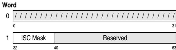
2. Control register 6 is set to all zeros during initial CPU reset.
