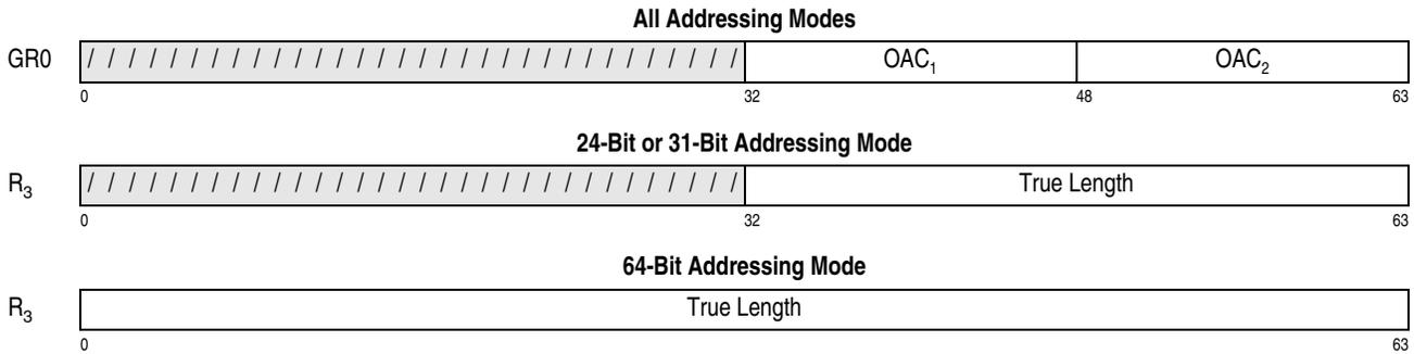
Figure 10-35. Register Contents for MOVE WITH OPTIONAL SPECIFICATIONS
