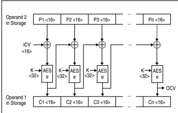
Figure 7-70. KMC AES Encipher Operation Using 256-Bit Key
