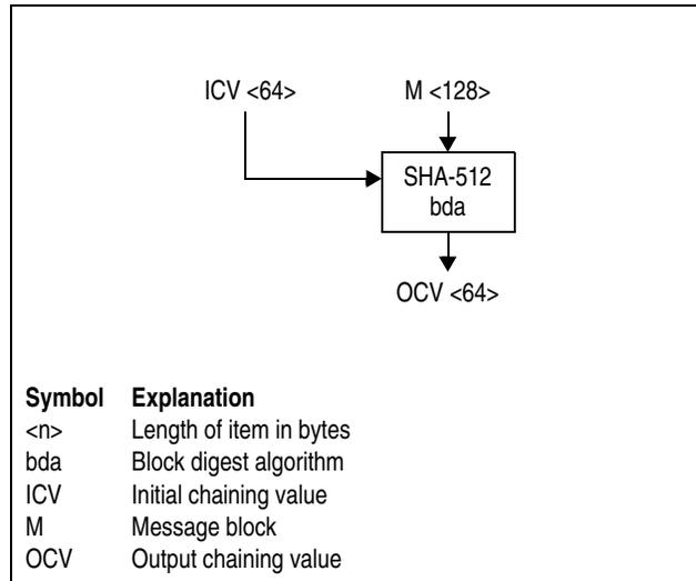
Figure 7-211. Symbol for SHA-512 Block Digest Algorithm
