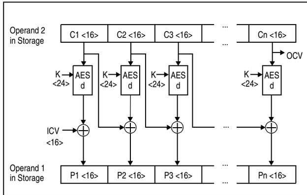
Figure 7-67. KMC AES Decipher Operation Using 192-Bit Key
