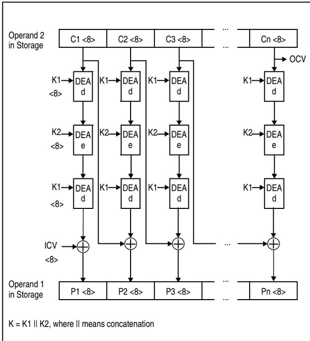
Figure 7-55. KMC TDEA Decipher Operation Using 128-Bit Key
