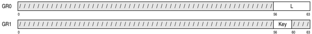
Figure 10-32. Register Contents of MOVE WITH DESTINATION KEY
