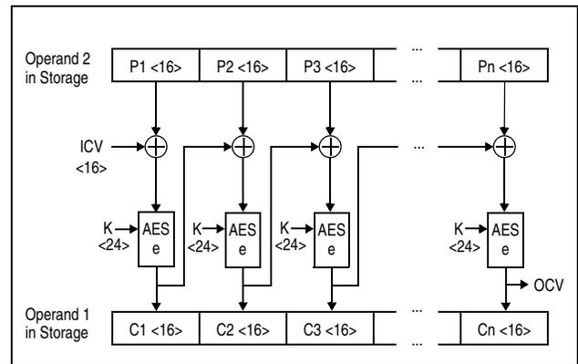
Figure 7-66. KMC AES Encipher Operation Using 192-Bit Key
