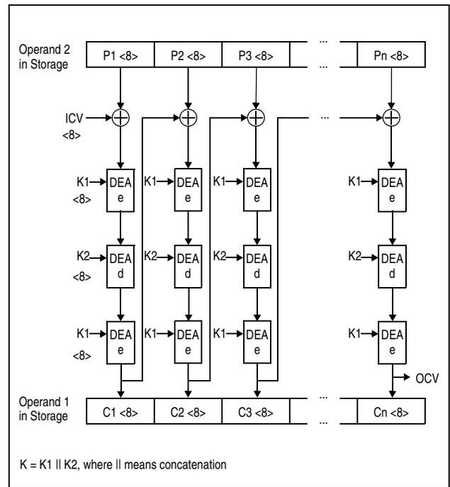
Figure 7-54. KMC TDEA Encipher Operation Using 128-Bit Key
