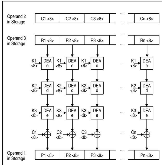
Figure 7-144. KMCTR TDEA Decipher Operation Using 192-Bit Key
