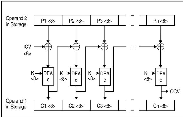
Figure 7-50. KMC DEA Encipher Operation Using 64-Bit Key
