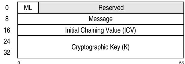
Figure 7-317. Parameter Block for PCC-Compute-Last-Block-CMAC-Using-TDEA-128
