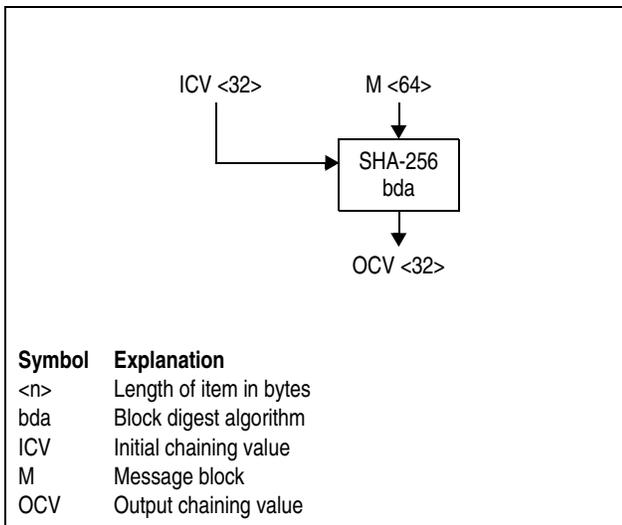
Figure 7-210. Symbol for SHA-256 Block Digest Algorithm
