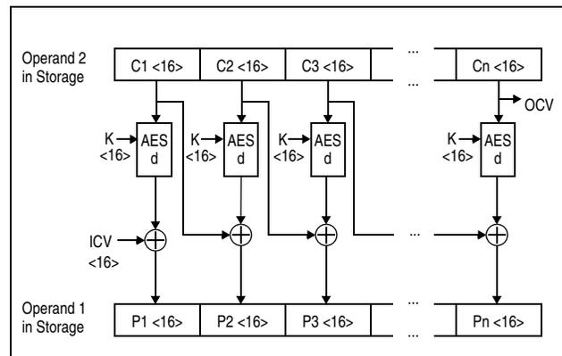
Figure 7-63. KMC AES Decipher Operation Using 128-Bit Key
