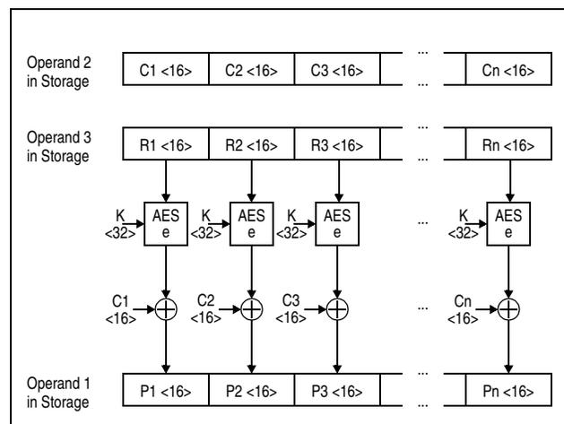
Figure 7-156. KMCTR AES Decipher Operation Using 256-Bit Key
