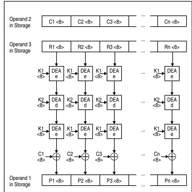
Figure 7-140. KMCTR TDEA Decipher Operation Using 128-Bit Key
