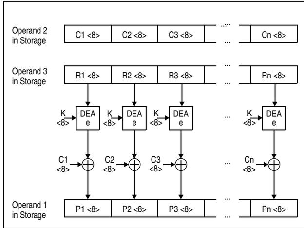
Figure 7-136. KMCTR DEA Decipher Operation Using 64-Bit Key
