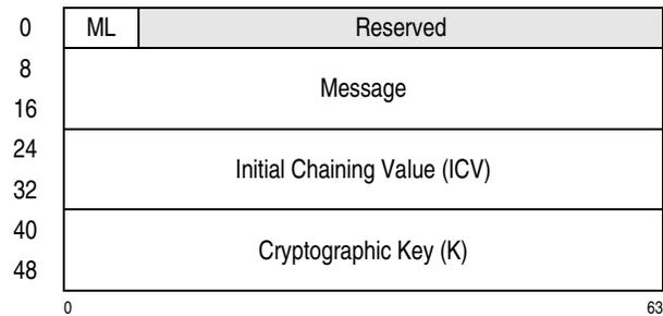
Figure 7-323. Parameter Block for PCC-Compute-Last-Block-CMAC-Using-AES-128
