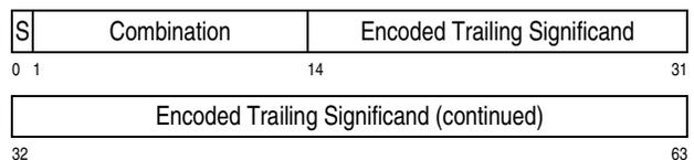
When an operand in the DFP long format is loaded into a floating-point register, it occupies the entire register.
