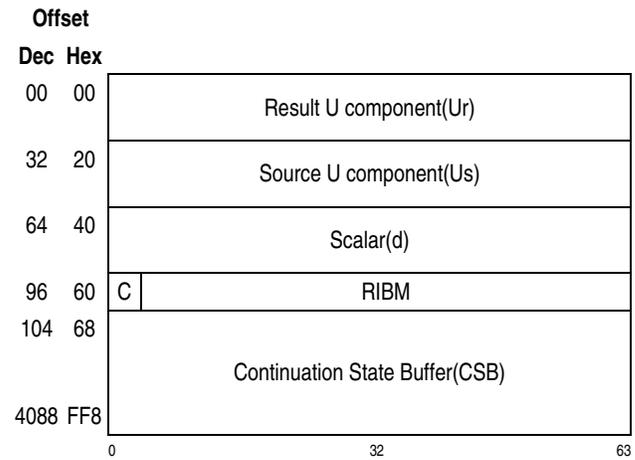
Figure 7-342. Parameter Block for PCC-Scalar-Multiply-X25519 Function
