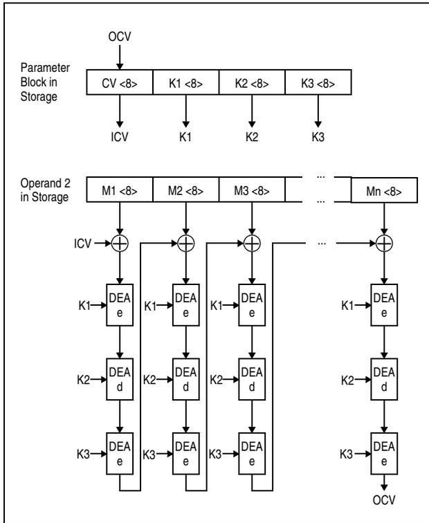
Figure 7-282. MAC Computation Using 192-bit TDEA Key
