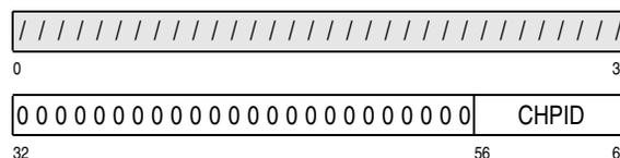
**Channel-Path Identifier (CHPID):** Bit positions 56-63 of general register 1 contain an unsigned binary integer that designates the channel path on which the channel-path-reset function is to be performed.
