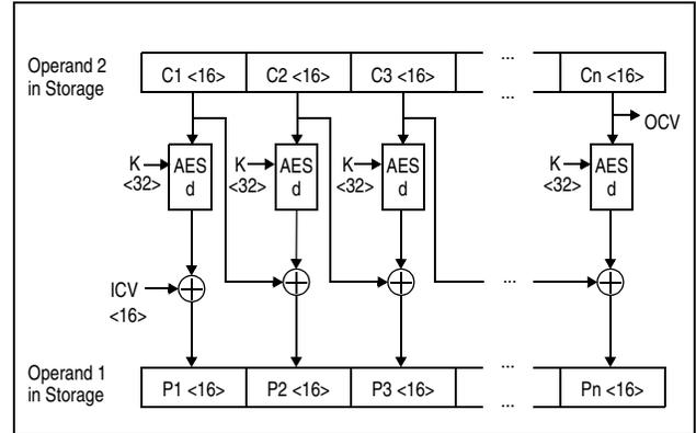
Figure 7-71. KMC AES Decipher Operation Using 256-Bit Key
