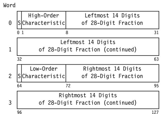
An HFP number has two signs: one for the fraction and one for the exponent. The fraction sign, which is also the sign of the entire number, is the leftmost bit of each format (0 for plus, 1 for minus). The numeric part of the fraction is in true notation regardless of the sign. The numeric part is contained in bits 8-31 for the short format, in bits 8-63 for the long format, and in bits 8-63 followed by bits 72-127 for the extended format.
