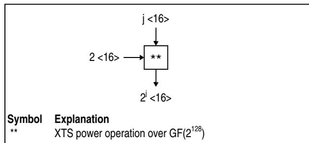
Figure 7-308. Symbol For XTS Power Operation Over  $GF(2^{128})$
