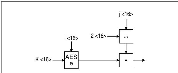
Figure 7-334. Compute XTS Parameter Using AES 128
