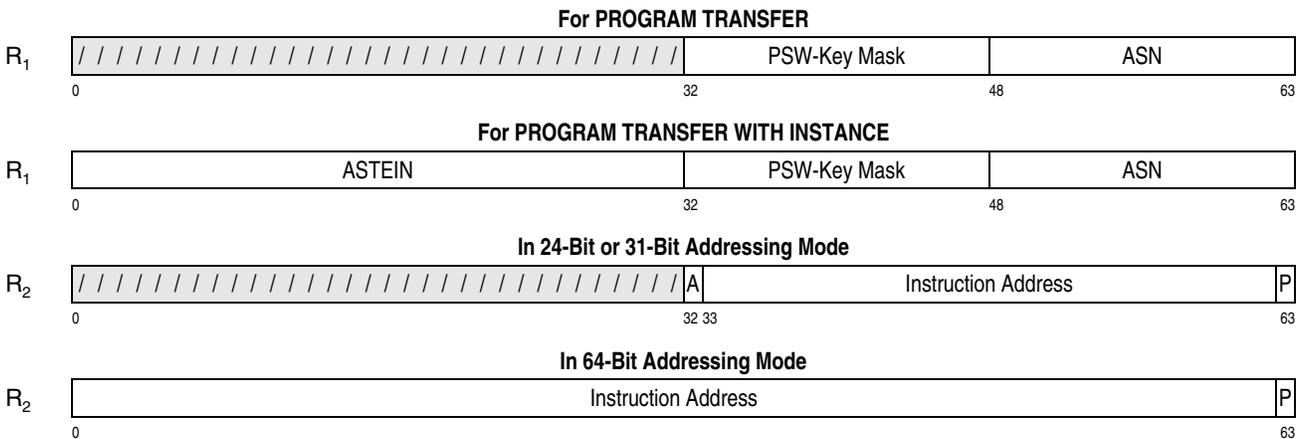
Figure 10-74. Register Contents for PROGRAM TRANSFER (WITH INSTANCE)
