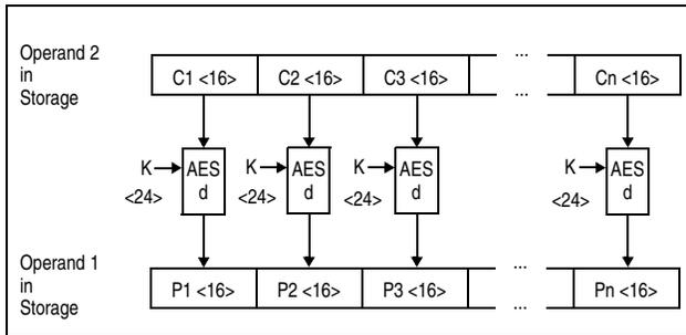
Figure 7-34. KM AES Decipher Operation Using 192-Bit Key
