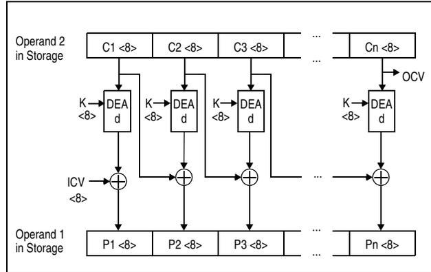
Figure 7-51. KMC DEA Decipher Operation Using 64-Bit Key
