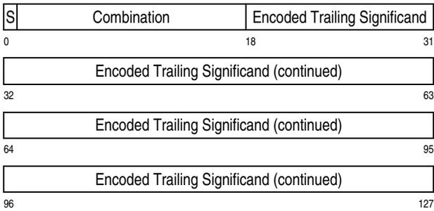
An operand in the DFP extended format occupies a register pair. The leftmost 64 bits occupy the entire lower-numbered register of the pair and the rightmost 64 bits occupy the entire higher-numbered register.
