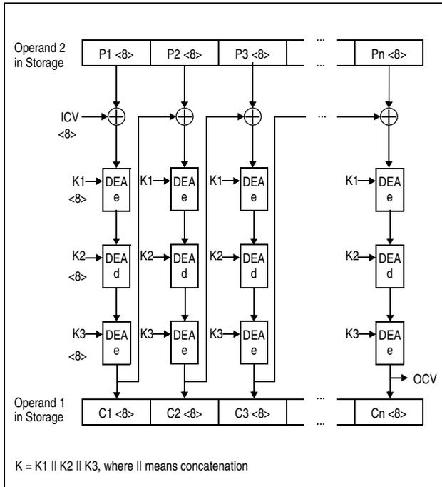
Figure 7-58. KMC TDEA Encipher Operation Using 192-Bit Key
