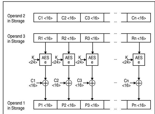
Figure 7-152. KMCTR AES Decipher Operation Using 192-Bit Key
