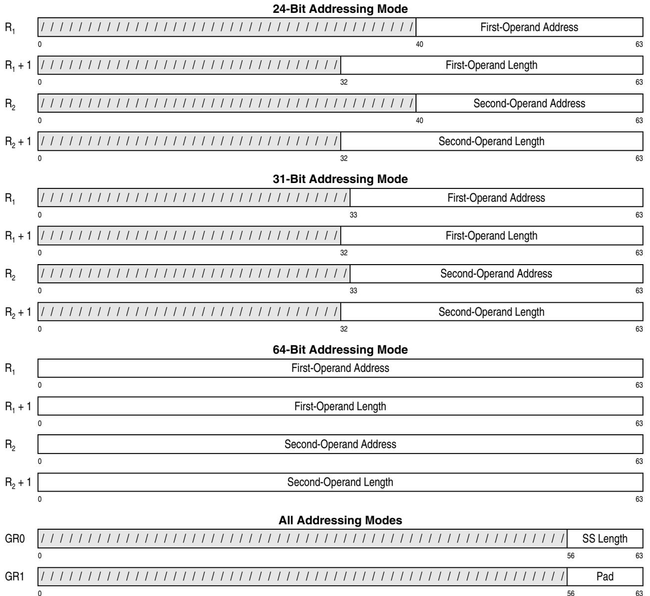
Figure 7-199. Register Contents for COMPARE UNTIL SUBSTRING EQUAL
