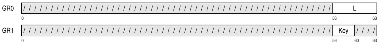
Figure 10-37. Register Contents of MOVE WITH SOURCE KEY
