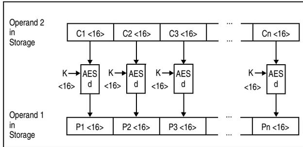
Figure 7-30. KM-AES Decipher Operation Using 128-Bit Key
