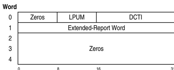
**Last-Path-Used Mask (LPUM):** For a definition of the LPUM, see “Last-Path-Used Mask (LPUM)” on page 16-49.
