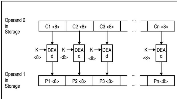
Figure 7-18. KM-DEA Decipher Operation Using 64-Bit Key
