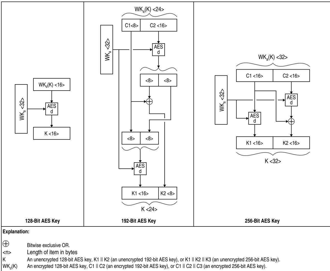
Figure 7-377. Decryption of AES Keys Using WK<sub>d</sub>
