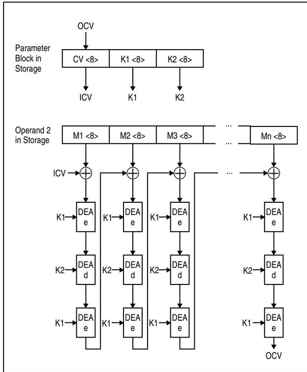
Figure 7-279. MAC Computation Using 128-bit TDEA Key
