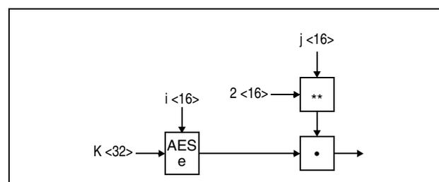
Figure 7-337. Compute XTS Parameter Using AES 256
