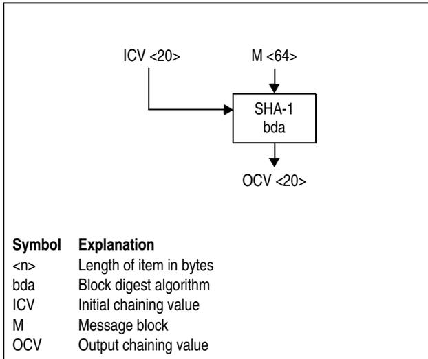
Figure 7-209. Symbol for SHA-1 Block Digest Algorithm
