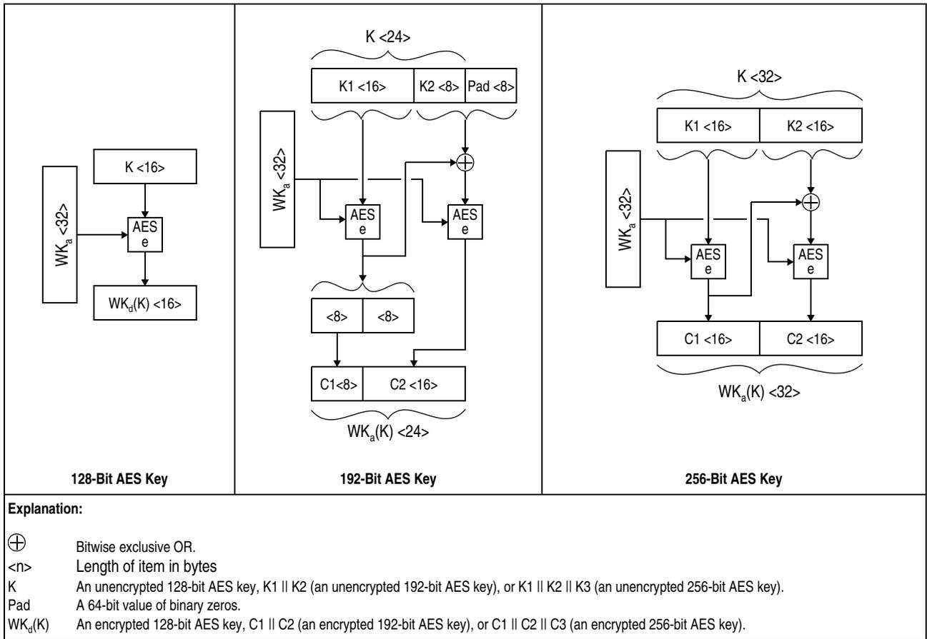
Figure 7-376. Encryption of AES Keys Using  $WK_d$
