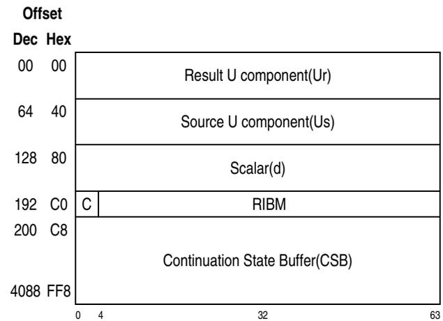
Figure 7-343. Parameter Block for PCC-Scalar-Multiply-X448 Function
