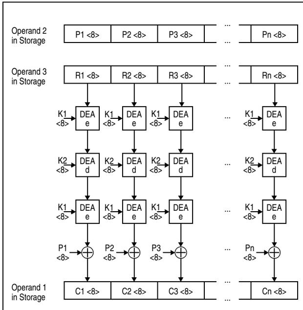
Figure 7-139. KMCTR TDEA Encipher Operation Using 128-Bit Key
