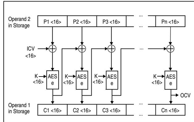
Figure 7-62. KMC AES Encipher Operation Using 128-Bit Key
