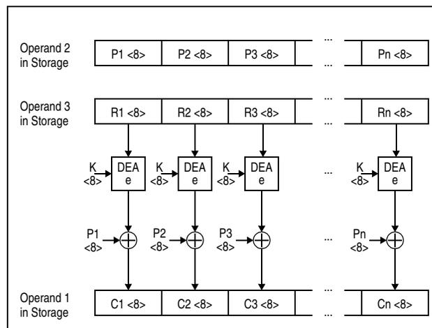
Figure 7-135. KMCTR DEA Encipher Operation Using 64-Bit Key
