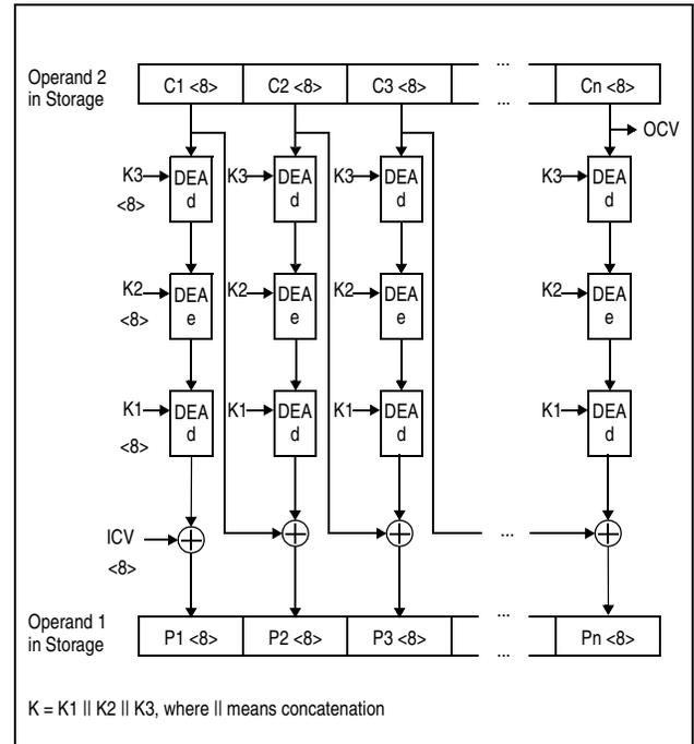
Figure 7-59. KMC TDEA Decipher Operation Using 192-Bit Key
