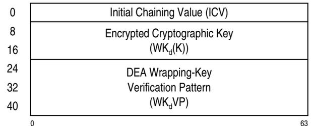
Figure 7-278. Parameter Block for KMAC-Encrypted-TDEA-128
