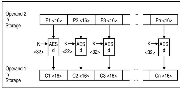
Figure 7-38. KM AES Decipher Operation Using 256-Bit Key
