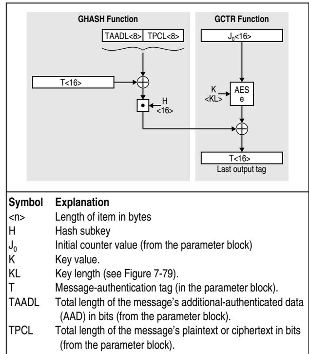
Figure 7-89. Hashing and Encrypting the Last Tag
