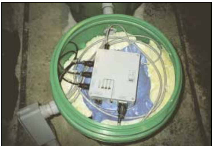
Figure 13. Seismometer feedback electronics connected to seismometers.
