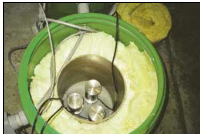
Figure 8. Guralp CMG-3NSN seismometers installed.
