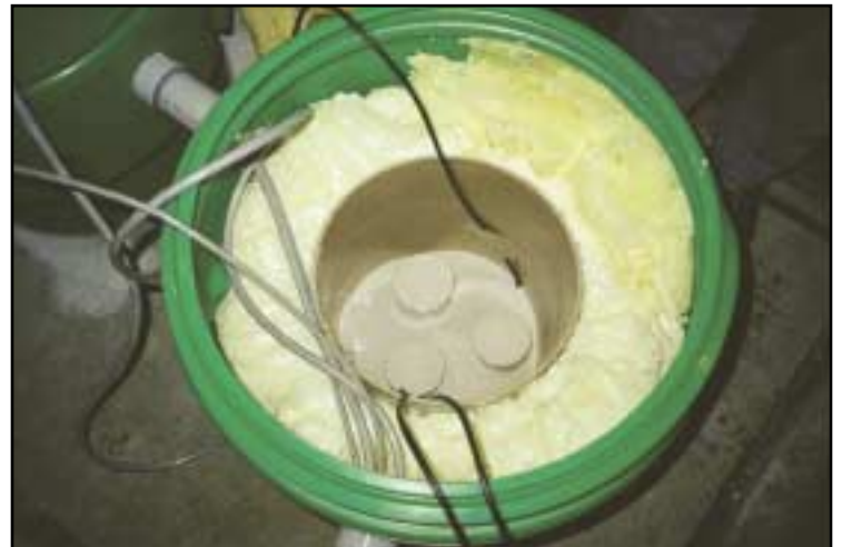
Figure 10b. Sand will completely cover seismometers when finished.
