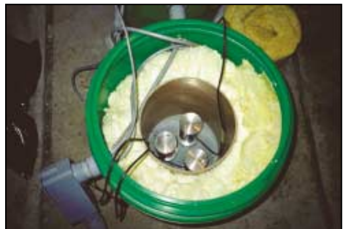
Figure 6. Polyurethane insulation in place.
