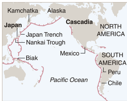
Subduction zone Line shows upper edge of plate-boundary fault. Teeth point down fault (p. 8).
