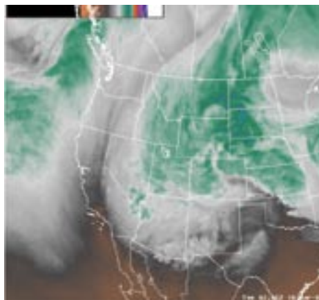
Figure 5. GOES, 6.7 μm water vapor image taken at 7:45 pm on 17 March 2003. The image shows the moisture associated with the warm conveyor belt stretching from northeastern Oklahoma, across most of Kansas, and westward into northern Colorado. At this time the surface low pressure is moving into southeast Colorado.
