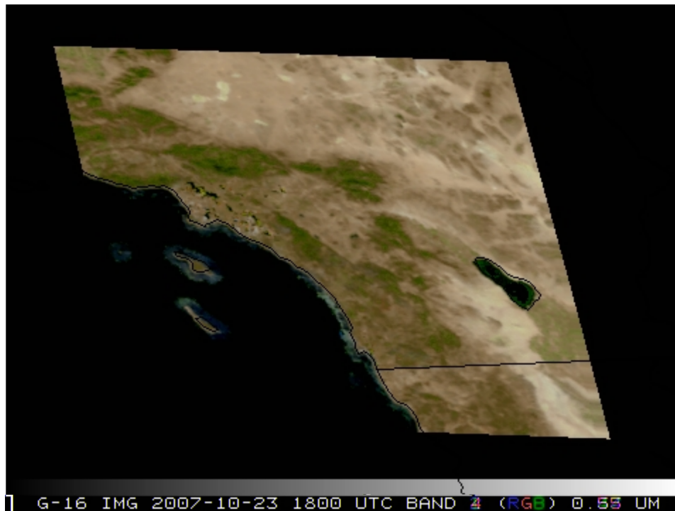
Fig. 2 Natural color image of the cloud-free 23 October 2007 southern California case, at 1800 UTC, using a look-up table green reflectance values from Eq. (1).
