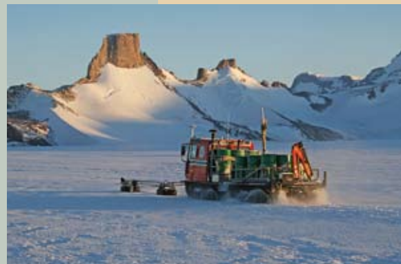
Figure 2. Crevasse detection using a vehicle-mounted radar system; Stabben is the mountain in the background, near Troll Station. (Photo: G. Liston)
