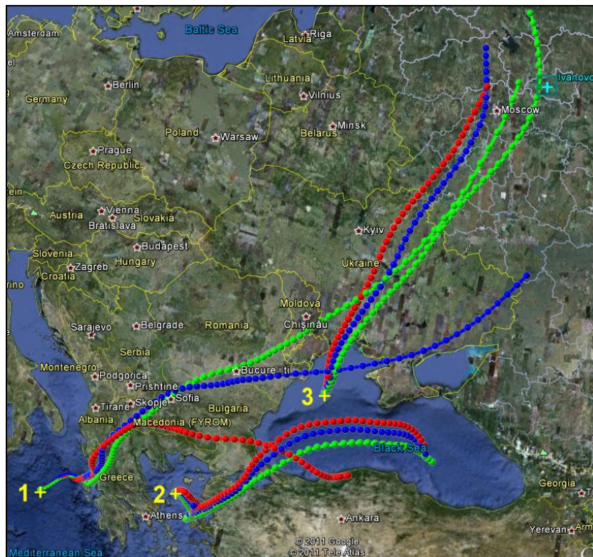
Figure 12. HYSPLIT forward trajectories with starting locations indicated by yellow + symbols. Initial times and number of hours run for source region 1) 1200 UTC 5 June, 96 h, 2) 1200 UTC 6 June, 72 h, 3) 1200 UTC 7 June, 48 h. Location of Ivanovo indicated by the cyan + symbol. Initial trajectory heights are 100 m (red), 250 m (blue), 500 m (green) AGL. Background image courtesy Google. Click image to enlarge.
