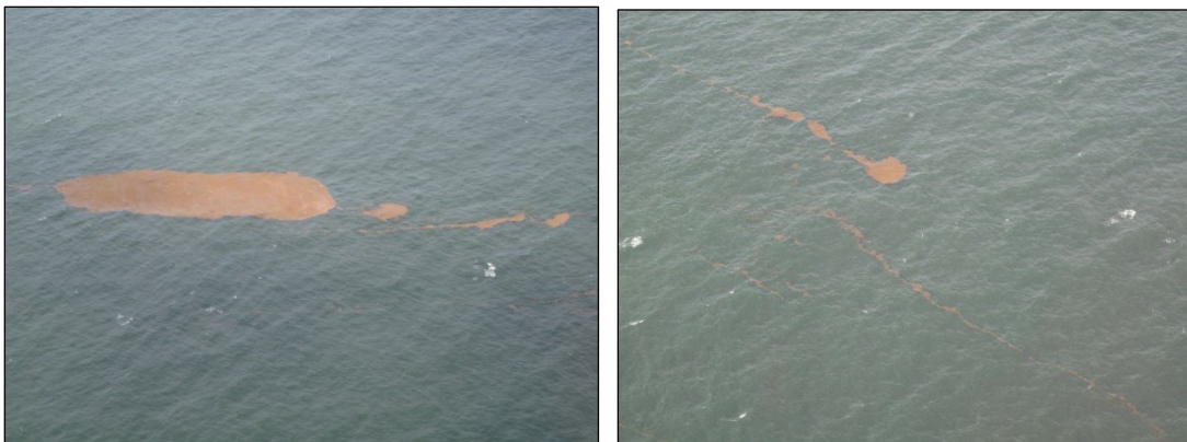
Figure 3-3. Example overflight photos of uniled Sargassum as false positives for floating emulsified oil. Photo credit: David Wesley/NOAA.
