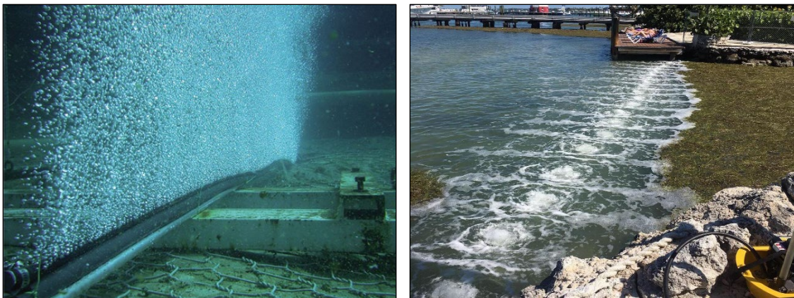
Figure 3-6. Bubble curtains underwater (left) and installed at the mouth of a canal, preventing seaweed from crossing the barrier (right). Source: https://www.diversifiedpondsupplies.com/bubble-tubing/bubble-curtain and https://flkeysaeration.com/wp-content/uploads/2019/01/Marathon-Bubble-Curtain-011319-6.jpg .
