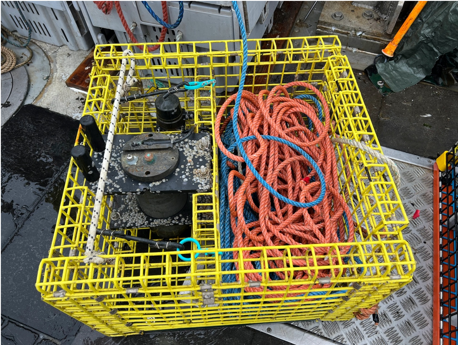
EdgeTech inshore cage, with lid removed. Acoustic release on left, coiled endline on right.
