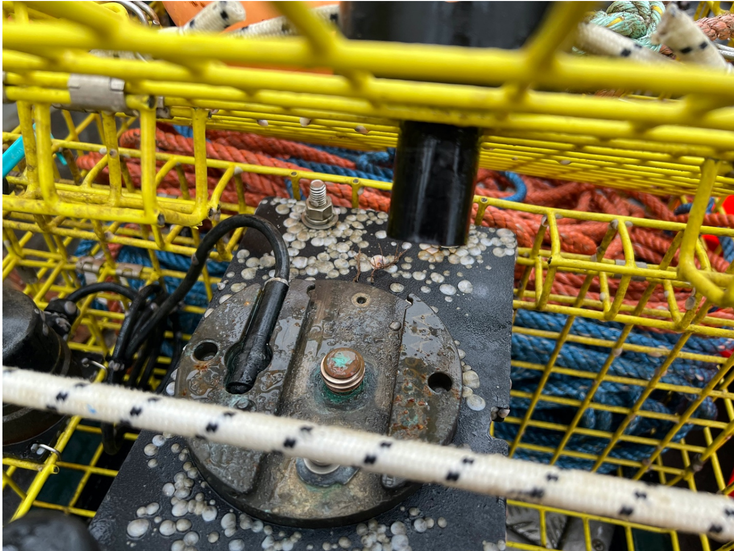
Detail of the acoustic release in an EdgeTech unit. The threaded spindle is acoustically triggered to rotate until the threaded coupling in the black puck above is released, allowing the buoyant lid to ascend. This unit has been deployed multiple times and has evidence of fouling.
