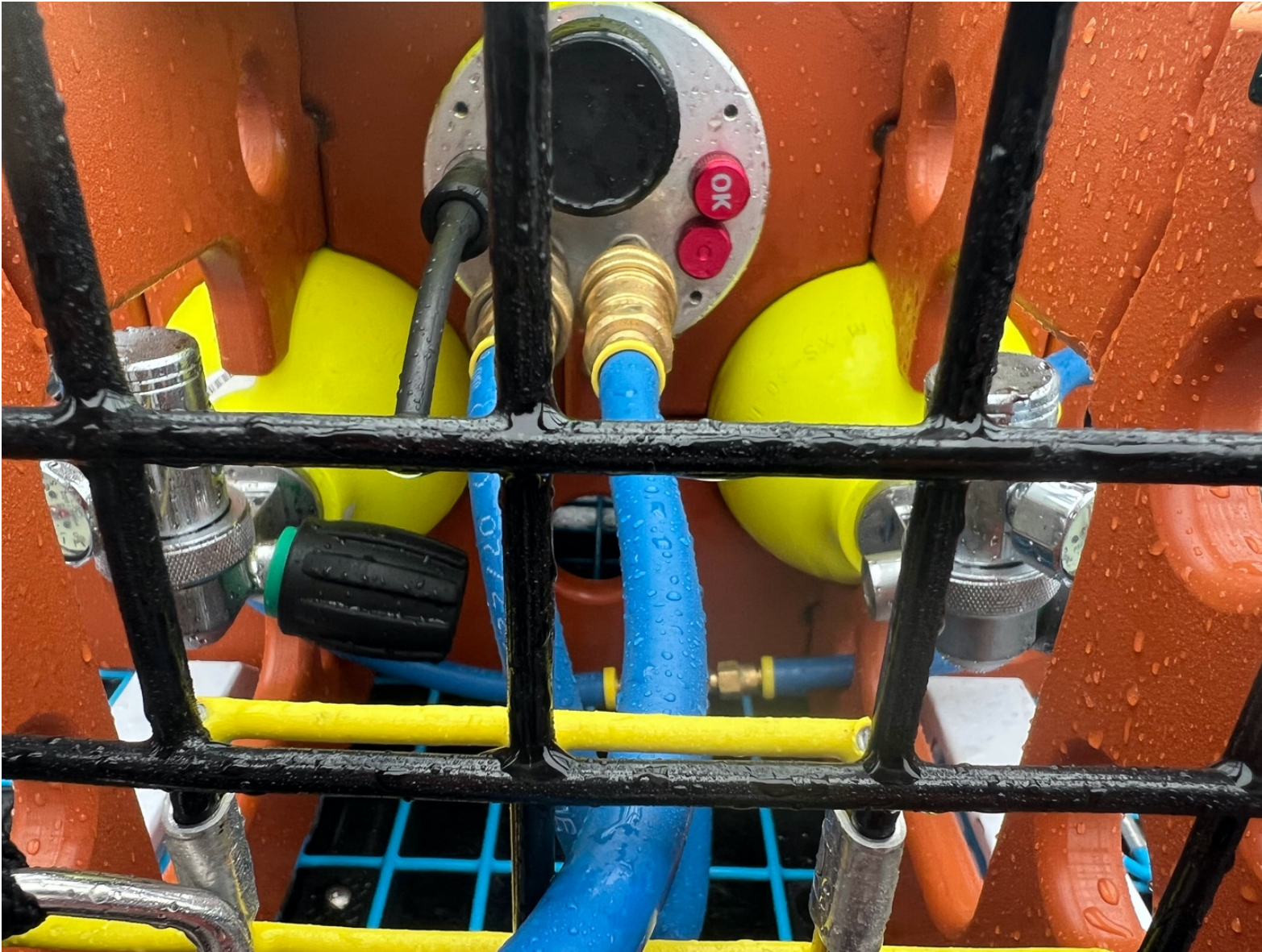
SMELTS – Detail of the two air tanks, and acoustic triggered release valve.
