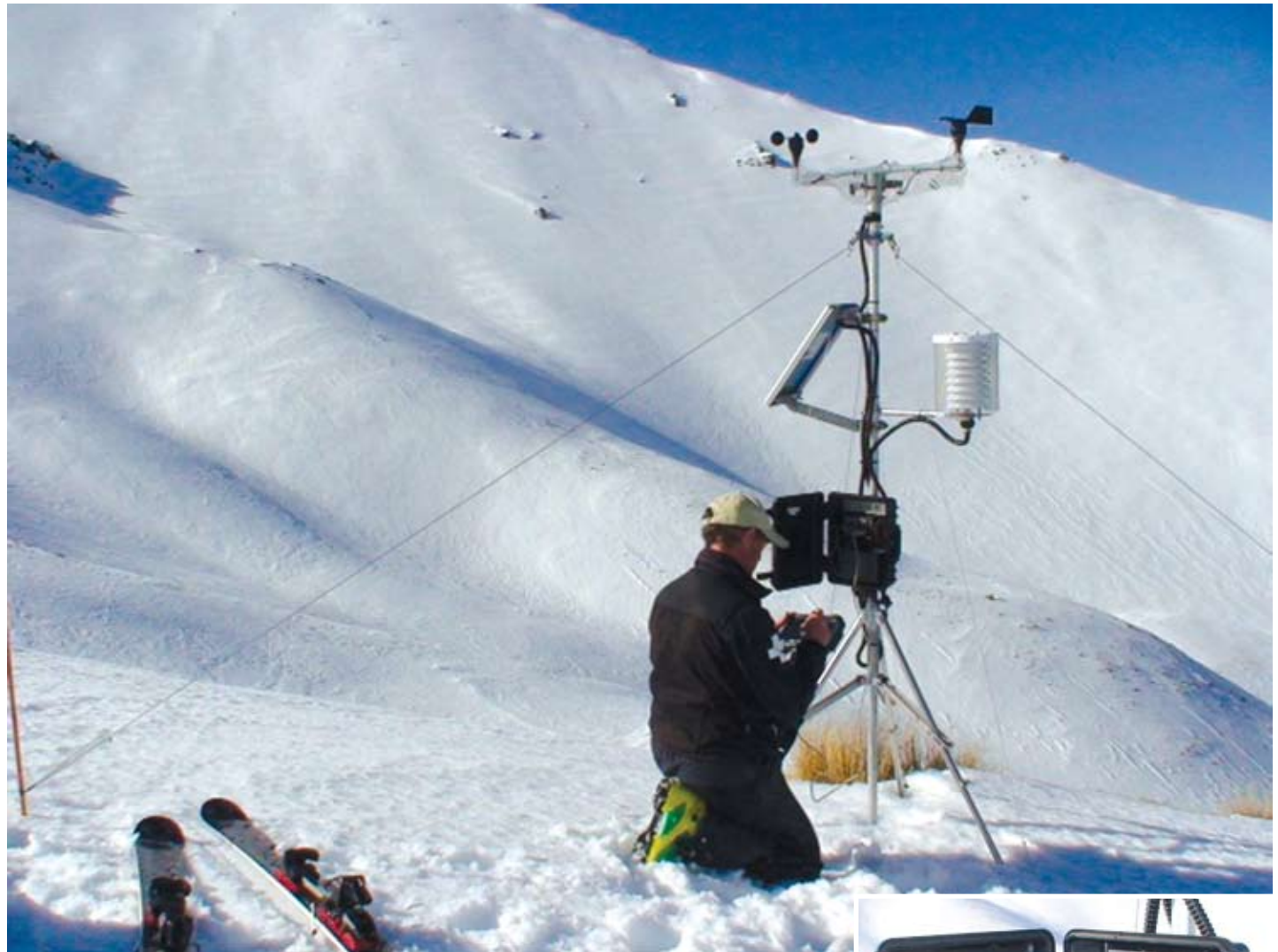
Downloading meteorological data from one of the Crystal Valley automatic weather stations with the Trimble rugged tablet computer (close up, right).
