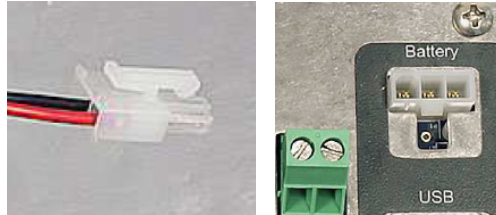
FIGURE 8-8. –ALK Battery Pack Connector Cable and CRVW3 Battery Connection
