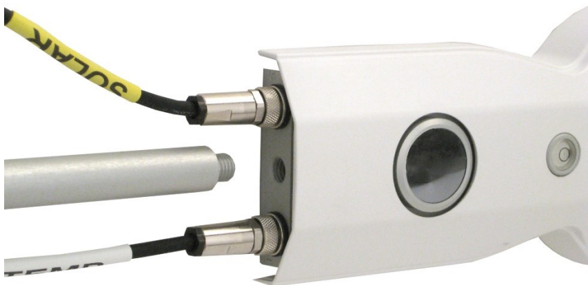
Figure 7-1. Attaching the mounting rod to the CNR4 body
