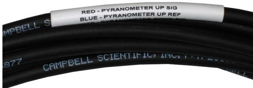
Figure 7-5. Labels on the pigtail end of the SOLAR cable
