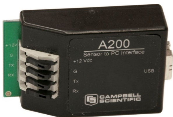
Figure 8-1. A200 Sensor-to-Computer Interface
