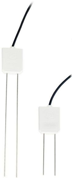
Figure 5-1. CS650 (left) and CS655 Water Content Reflectometers
