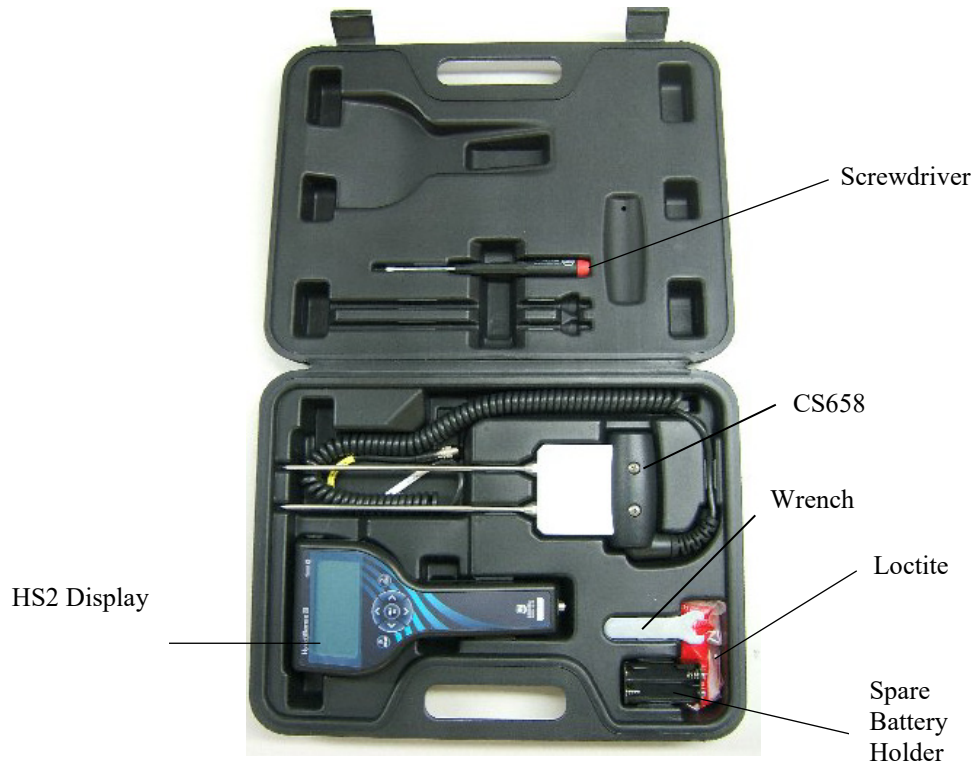
FIGURE 4-1. HS2 Parts in Hard Carrying Case
