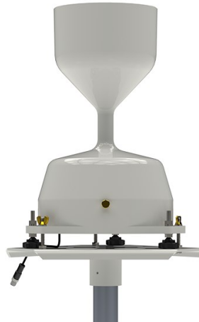
Figure 7-8. RainVUE-series mounted on a pole
