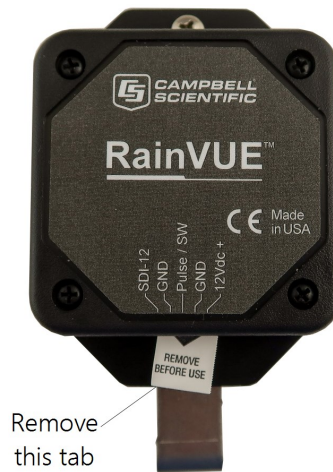
Figure 7-7. RainVUE-series interface and insulator tab
