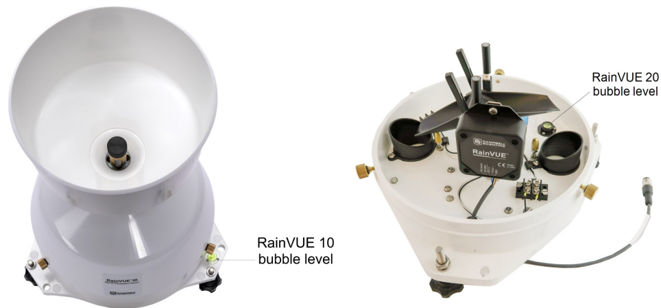
Figure 7-6. Bubble level locations on the RainVUE-series
