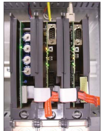
Figure 2. To wire the BCM-PWS (left), BCM-ETH (center), and BCM-MDBS (right), lift their hinged lids. Wire them in series.
