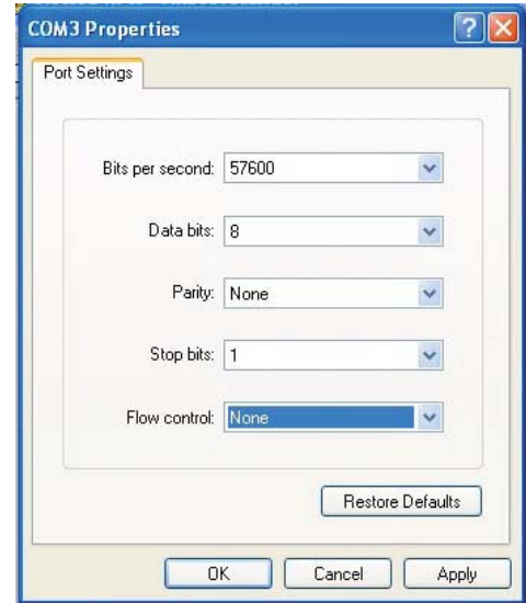
Figure 5: HyperTerminal Port settings.
