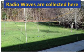
Dual Dipole Radio Antenna 12 m (40 ft) x 9 m (30 ft)
