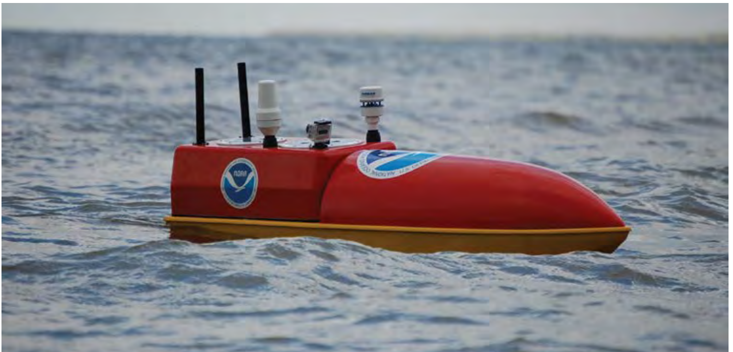
EMILY (an acronym for Emergency Integrated Life Saving Lanyard), a 65-inch water-tight craft, is one of NOAA's hurricane research platforms. Outfitted with a satellite link, camera, battery and gasoline motor, and a variety of sensors, EMILY will collect sea-level data from within a hurricane. Credit: Hydronalix Inc.
