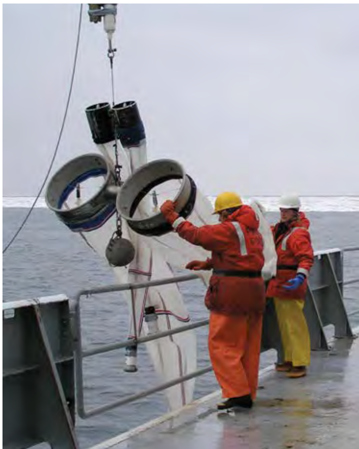
Nancy Kachel and Carol Ladd deploy a bongo net to sample for zooplankton at the ice edge in the Bering Sea aboard the Research Vessel Thomas G. Thompson. Kachel is with the NOAA Joint Institute for the Study of the Atmosphere and Ocean at the University of Washington. Ladd is with the NOAA Pacific Marine Environmental Laboratory in Seattle. Credit: NOAA
