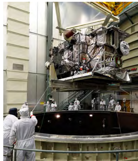
The GOES-17 satellite above the thermal vacuum chamber. Photo credit: Lockheed Martin.
